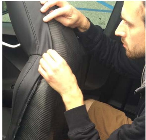
8. Press the trim strip firmly into the slot / seam around the seat back.
