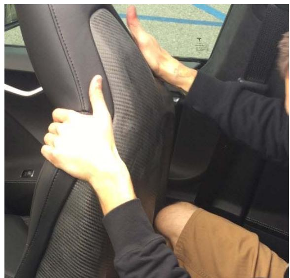
9. Continue pressing firmly around the perimeter of the seat to ensure the leather is fully tucked into its original position.
