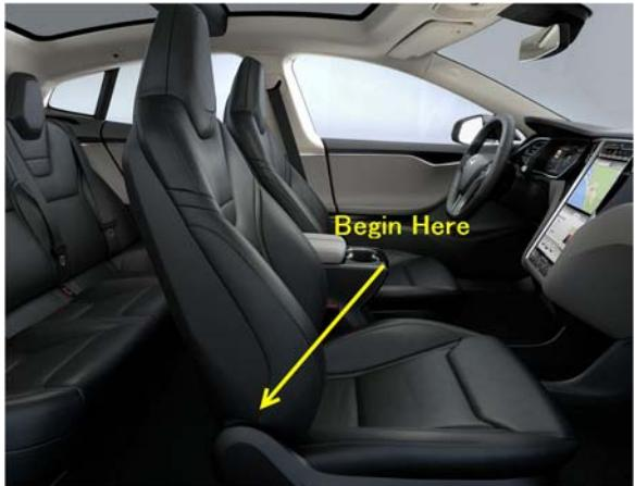
2. Make sure the pick is successfully hooked onto the leather, and begin to firmly pull to release the bead of plastic / rubber trim that holds the upholstery onto the seat frame.
